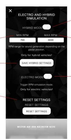
Minimum speed in E mode Value for idle speed of the simulated Active Sound noise in hybrid vehicles in electrical operation. It makes sense. For example 500 to 1000 revolutions per minute.
